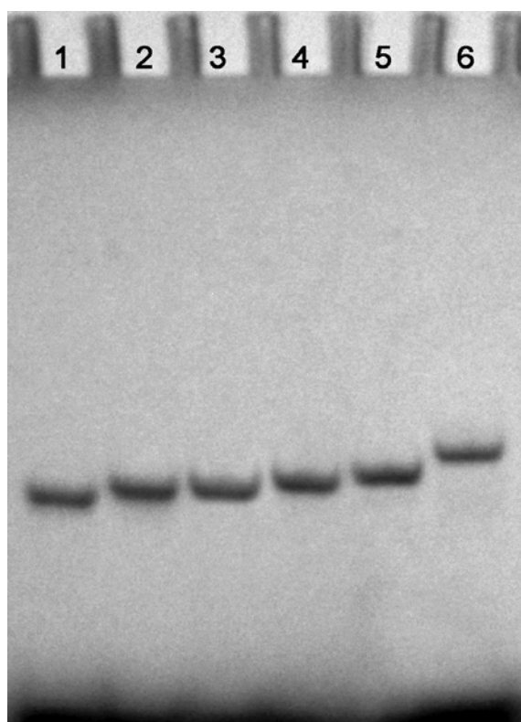
Figure 6.4. Non-denaturing 20% polyacrylamide gel of phenanthrene-containing hybrids. The line numbers correspond to the entry numbers in Table 6.1. , i.e. the number of phenanthrenes increases from left (zero) to right (seven). Bands were visualized by UV-light (260nm).
